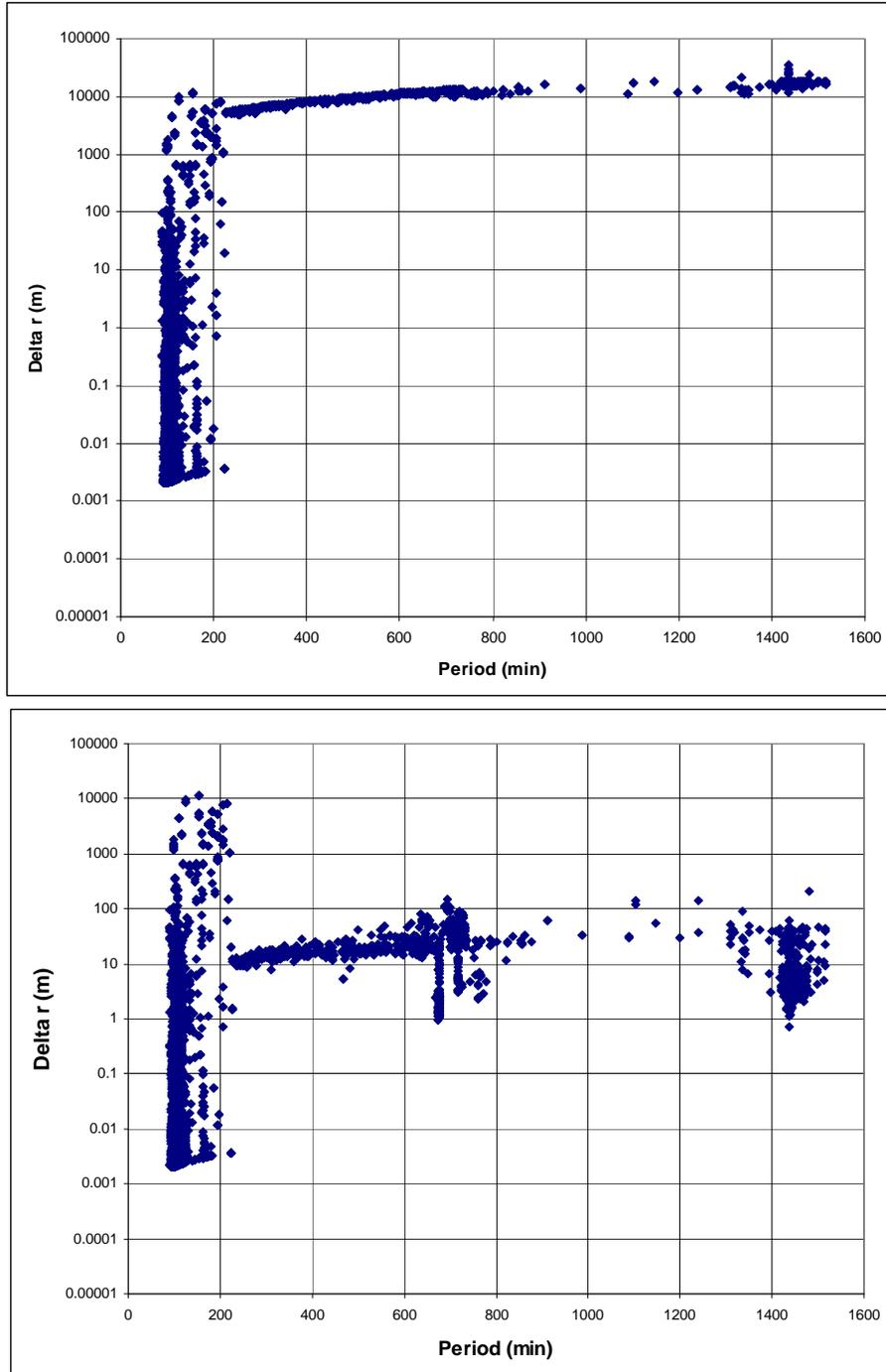
**Figure 10. SGP4 Full-Catalog Comparisons.** Maximum differences between ephemerides generated for 2 days are shown. The plot shows the paper C++ version against the original JPL code (plot on the top). Note that by changing the DOPERT variable in the JPL code, the results can be improved by about two orders of magnitude (plot on the bottom).
