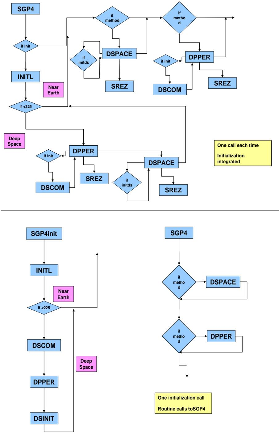
**Figure 4. SGP4 Structural Organization.** The computer program structure is shown for the original and derivative programs (top) and the revised version for this paper (bottom). Note that the initialization was interspersed throughout the original program, while it is better isolated in the revised code.
