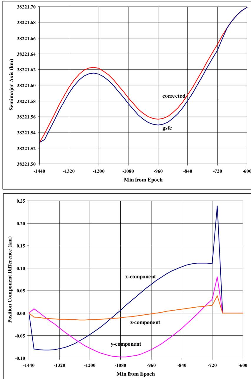
**Figure 6. Propagation Problems for Satellite 09998.** The integrator problem is shown by looking at the semimajor axis (top) and the positional component differences (bottom). The scale is small, but the semimajor axis clearly shows the jump caused by incorrect integrator performance near 720 minutes prior to the epoch. The problem appears in all older versions.
