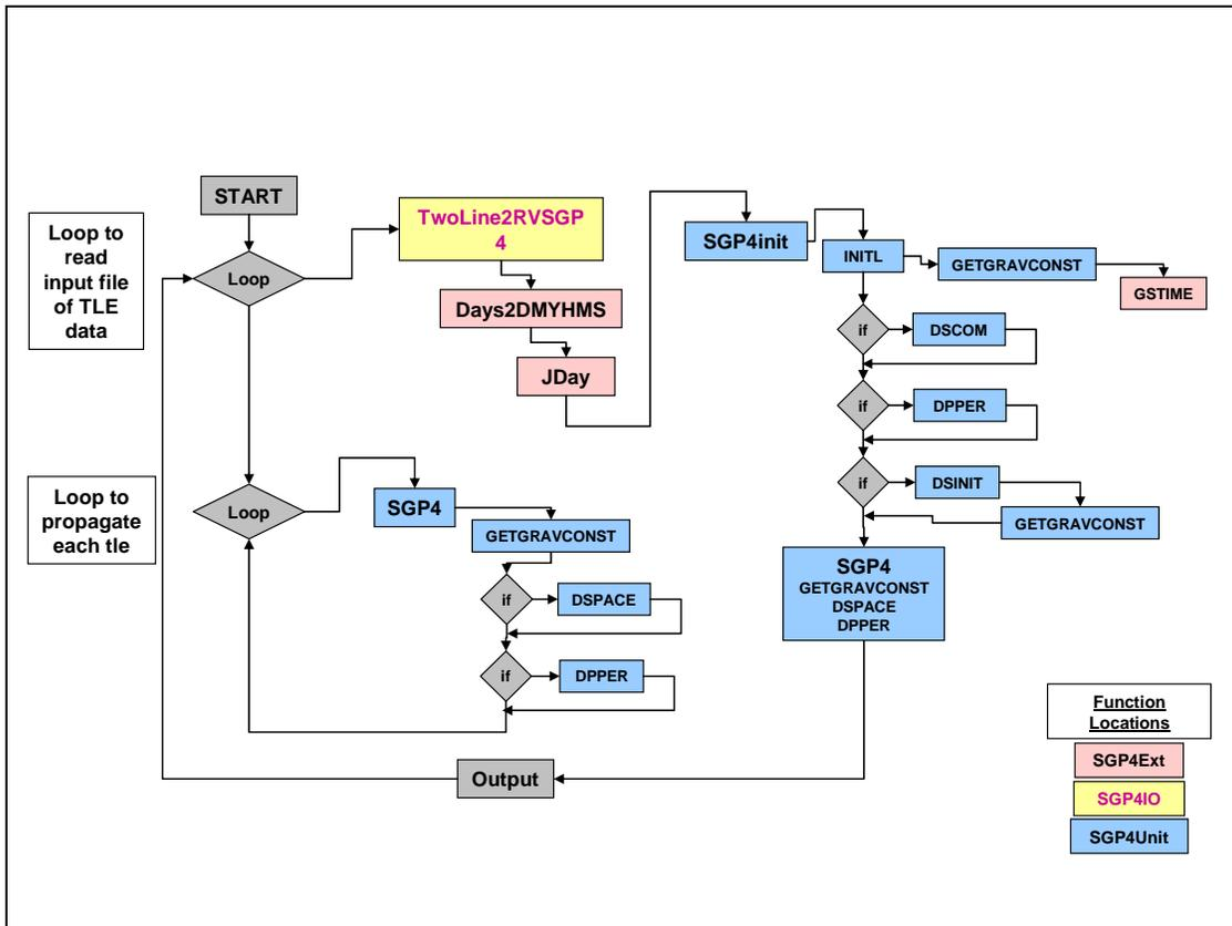
**Figure 12. Program Code Structure.** An example flowchart shows the relations between the various routines in the revised code. Note that the initialization is required a single time after each new TLE is processed.
