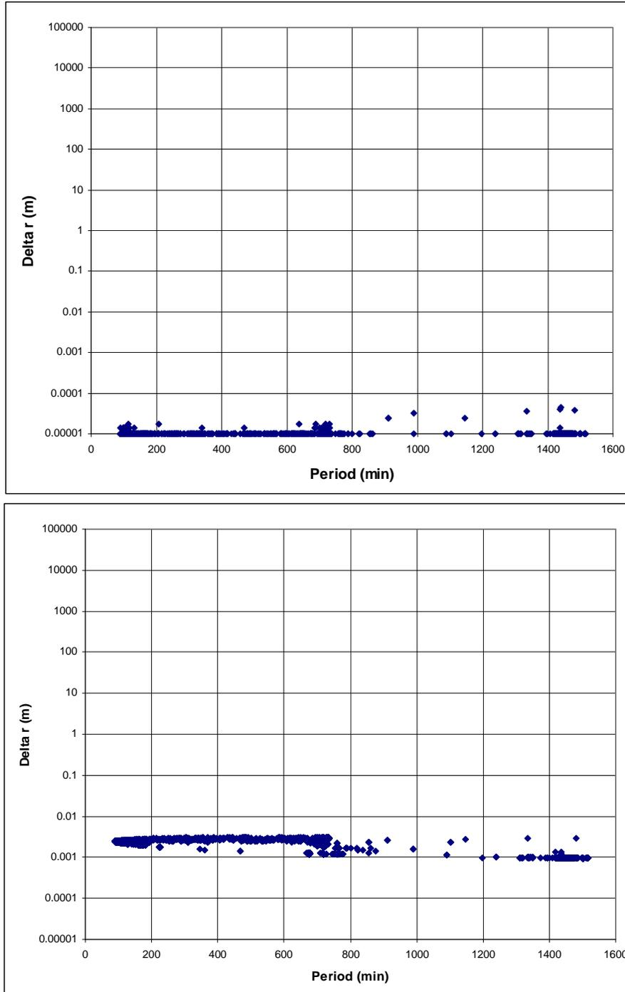
**Figure 7. SGP4 Full-Catalog Comparisons.** Maximum differences between ephemerides generated for two days are shown. Note the small scale for the C++ and FORTRAN comparison (top). The Pascal comparison (bottom) shows very small additional variations and these are from the 8-byte versus 10-byte precision in the language.
