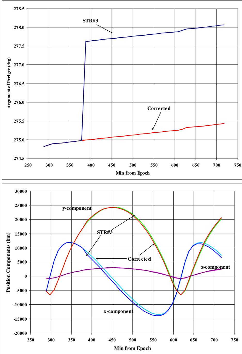
**Figure 2. Lunar-solar modifications for Satellite 23599.** The argument of perigee and positional components illustrate the discrepancy in incorrectly updating the lunar-solar perturbations, and not accounting for the proper quadrant in the periodic calculations. The problem existed in the STR#3 version, shown here, and an attempted correction was made in STR#6, but it was mostly corrected in the GSFC version.
