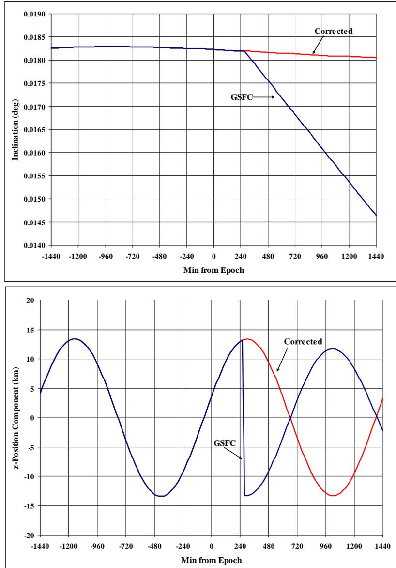
**Figure 5. Negative Inclination Performance for Satellite 25954.** The inclination and  $z$ -component of the position vector show the step function discontinuity of the previous SGP4 versions. The STR#3 and GSFC versions exhibits the problem while the Dundee version does not.
