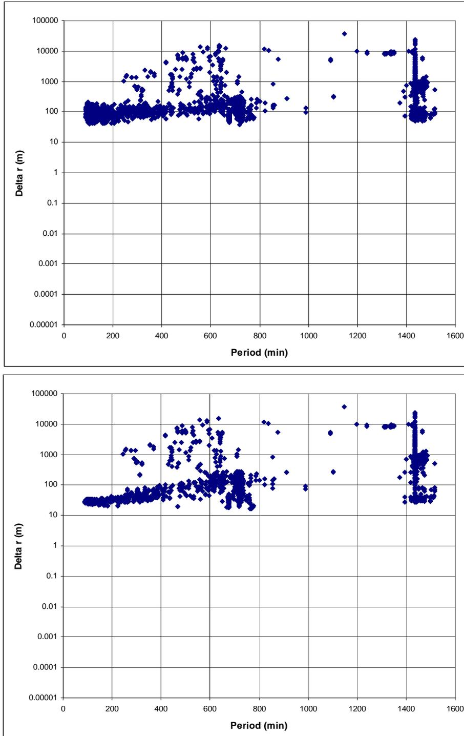
**Figure 9. SGP4 Full-Catalog Comparisons.** Maximum differences between ephemerides generated for 2 days are shown. The top plot shows the single-precision STR#3 version against the paper C++ version, while the bottom plot shows the STR#3 double-precision version comparison.
