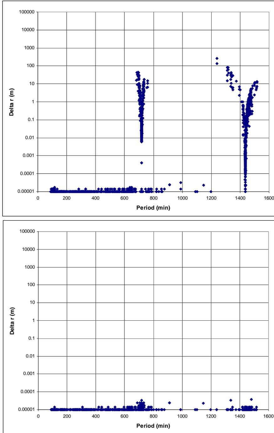
**Figure 8. SGP4 Full-Catalog Comparisons.** Maximum differences between ephemerides generated for 2 days are shown. The top plot shows the paper C++ version against the GSFC code, while the bottom plot shows the comparison to the GSFC code, but only for propagations positive from the epoch. The differences are all related to the integrator problems before 720 minutes prior to epoch with geosynchronous and semi-synchronous orbits.
