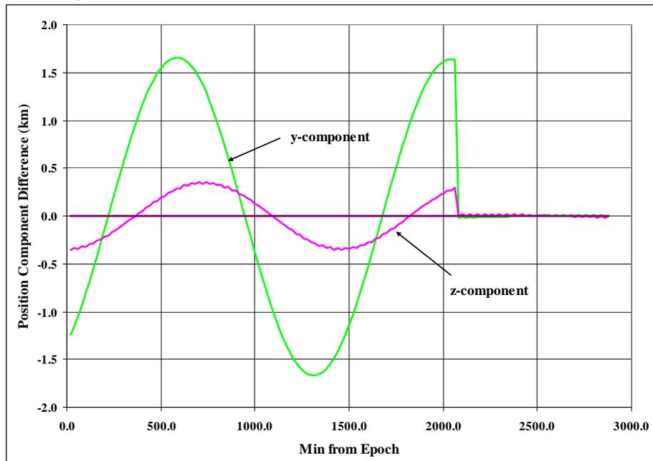
**Figure 3. Lyddane Choice Modification for Satellite 14128.** The difference in positional components illustrates the discrepancy in applying the Lyddane modification using the perturbed inclination rather than the original inclination. The effect exists when comparing the GSFC and STR#3 versions. Note the differences diminish once the inclination crosses the  $11.4592^\circ$  threshold (after 2000 min).
